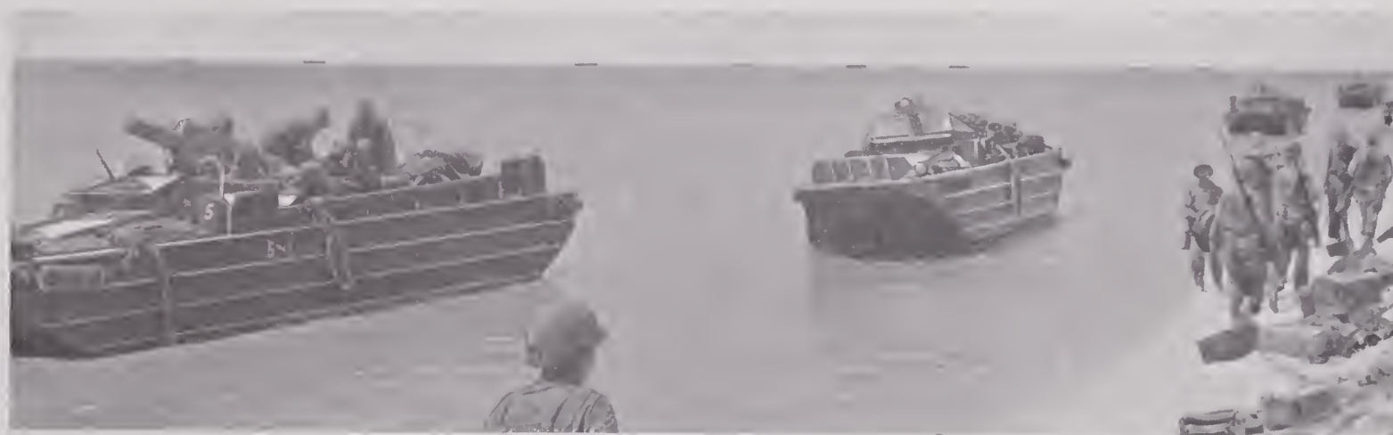
FIGURE 40. DUKWs at Saipan loaded with 105-mm howitzers and gun crews for invasion of Tinian Island.
